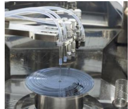
Developing Solvent & Aqueous Chemicals Spray and/or Puddle Process
